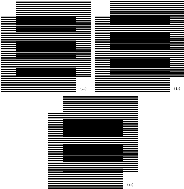
Figure 4. Superposition of two layers with parallel horizontal lines, where the revealing layer moves vertically at a slow speed [eps (a)] , [png (a)] , [eps (b)] , [png (b)] , [eps (c)] , [png (c)]
